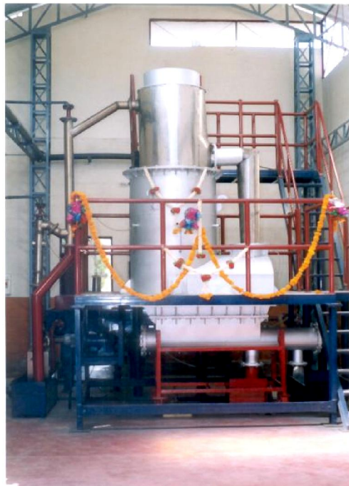
75 kg/hr gasifier system at NIE, Mysore
